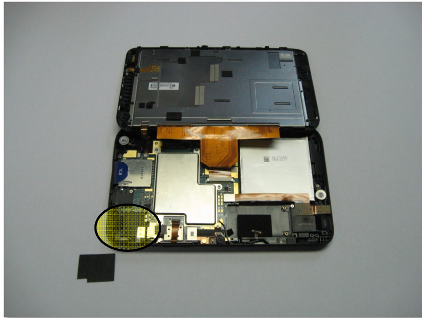
Figure 4 DELL STREAK 7 Tablet opened to locate the Wi-Fi antenna
